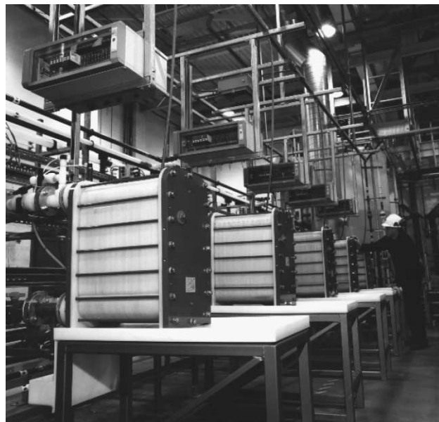
Fig. 3. Regenesys™ regenerative fuel cell modules.
